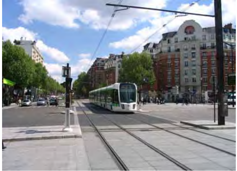
EXAMPLE OF AN "URBAN" LIGHT RAIL APPLICATION, WITH TRAINS RUNNING IN DEDICATED RIGHT-OF-WAY ALONG STREET CORRIDOR, AND MODERN LOW-FLOOR VEHICLES.
